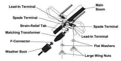
To connect coaxial cable to your antenna:
